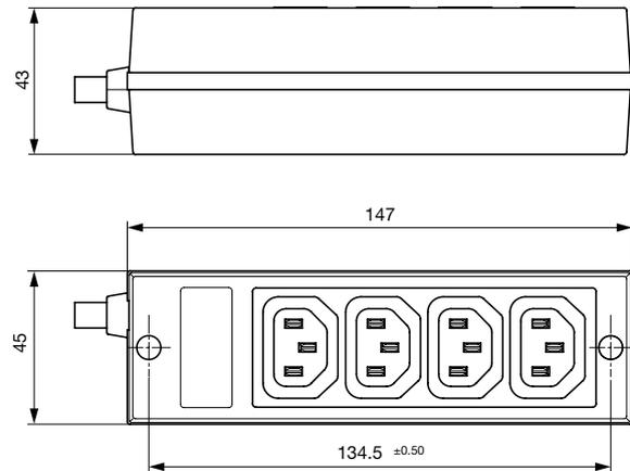
Mounting holes for 3 mm screws,
